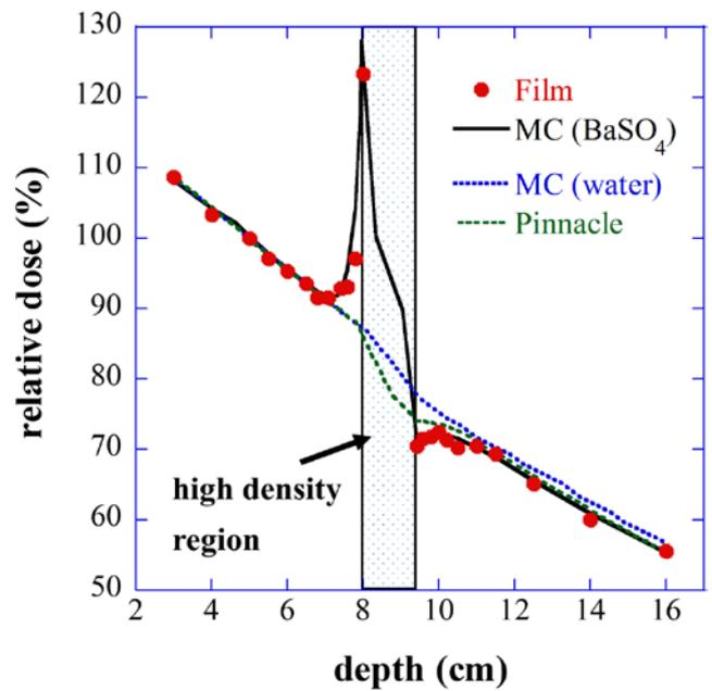
**Figure 4** : PDD calculated with each RTPS and measured with the use of EBT3 in a heterogeneous phantom. In the film measurement and MC simulation using BaSO<sub>4</sub>, the very high dose enhancement occurred proximal to the high density region. However, in the Pinnacle and MC simulation using water, dose enhancements were not found.
