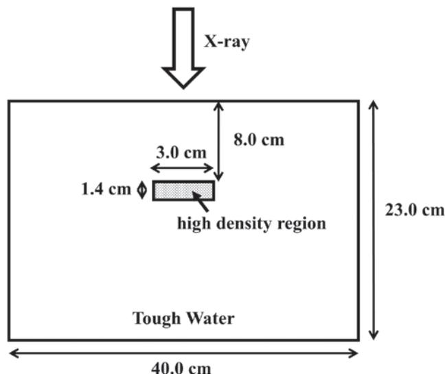
**Figure 1** : Measurement geometry. Tough Water Phantom and Neobalgin HD (a powdery contrast medium) were used. The field size was 10 cm x 10 cm at the isocenter, and SSD was 92 cm.
