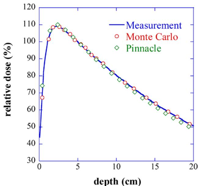
**Figure 3** : PDD calculated with each RTPS and measured with use of the ion chamber in water. With the exception of the build-up region, all relative errors were within 3%.
