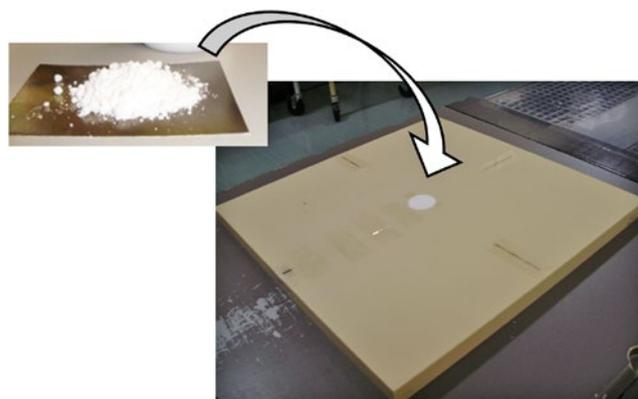
**Figure 2** : Creation of the high density region. The high density regions were created to fill the cavity for inserting the parallel plane type ion chamber in the Tough Water Phantom with contrast medium.
